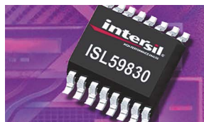
The latest ICs ease the task of analog-video-line driving and receiving: The Intersil ISL59830 triple driver requires no negative supply or blocking capacitors (left), and the Analog Devices AD8143 triple receiver lets systems operate with Category 5 twisted-pair cabling rather than more expensive cables (right).
